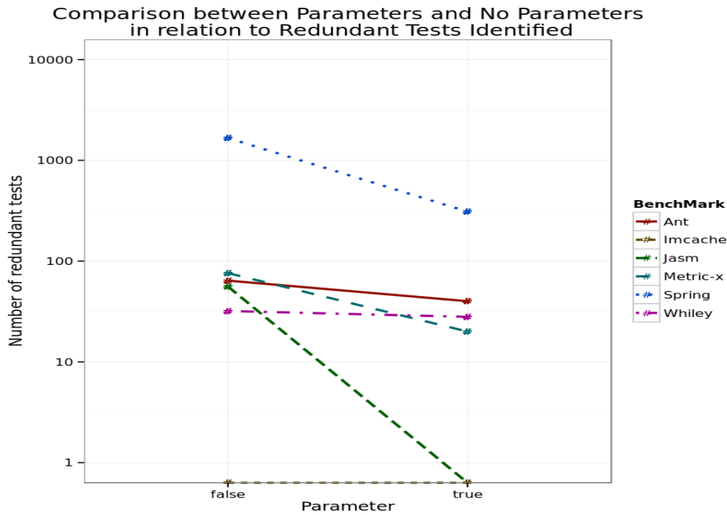
Figure 4.7: A figure showing the effect that using parameters has on the number of redundant tests are identified.
