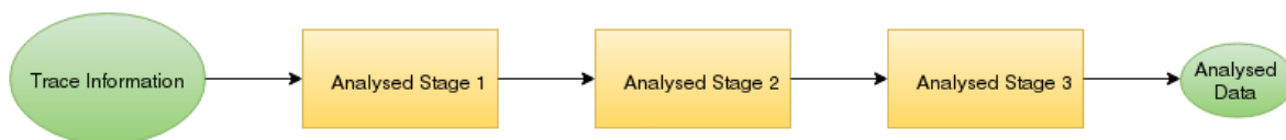
Figure 3.3: Trace information goes in at the start of the pipeline. After each stage there should be a reduction of comparisons that the next stage has to complete. The last stage should be the most computationally heavy.
