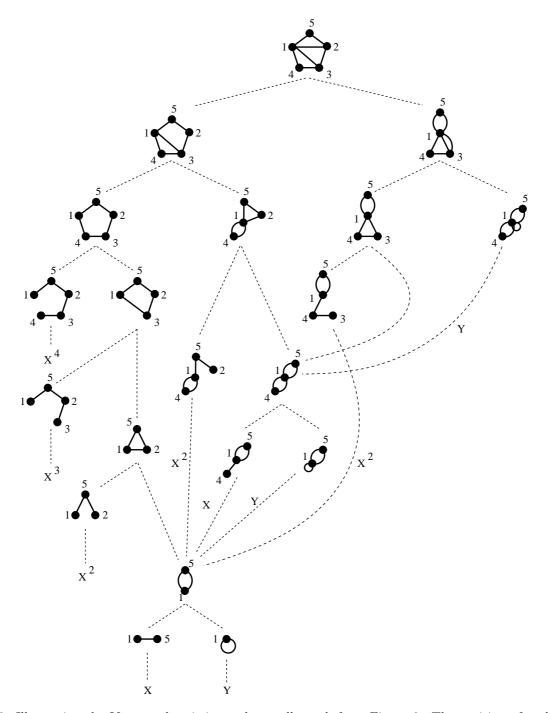
Figure 3: Illustrating the VORDER heuristic on the small graph from Figure 2. The position of each vertex in the order is shown next to it. Thus, the heuristic works aggressively on the vertex labelled 1, since this is lowest in the order.
