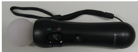
Figure 2.5: A PlayStation Move controller. Note the sphere (on the left) which can be lit up in a wide range of solid colours.
