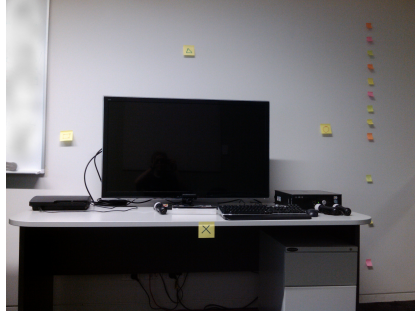
Figure 5.2: Experimental setup. The PlayStation eye camera is propped up on a book as the desk is too low. The vertical column of post-it notes contains measurements that participants could use to estimate their height.
