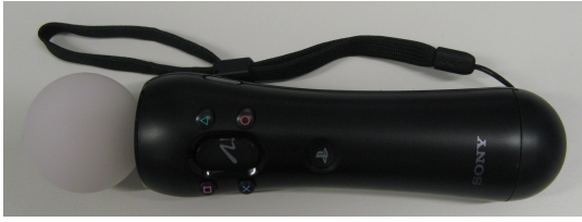
Figure 2: A PlayStation Move controller. The sphere (on the left) can be lit up in a range of solid colours
