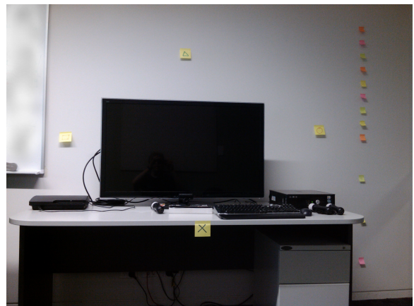
Figure 1: Experimental setup. The PlayStation eye camera is propped up on a book as the desk is too low. The vertical column of Post-it notes contains measurements that participants could use to estimate their height.
