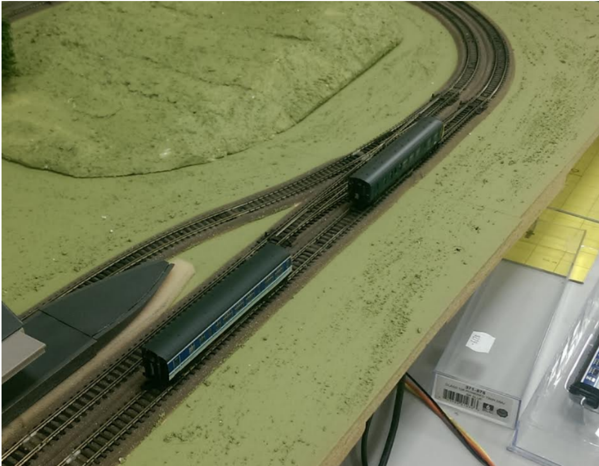
Figure 5.2: The trains on the model track one section behind the other. The locking controller should prevent a collision.
